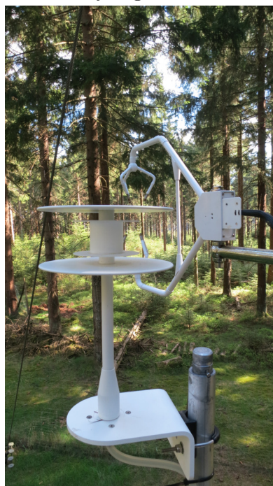
(D) Subcanopy measurement complex: Pressure port P3 (left) and CSAT3 (right) (photo: Laura Ehrnsperger).
