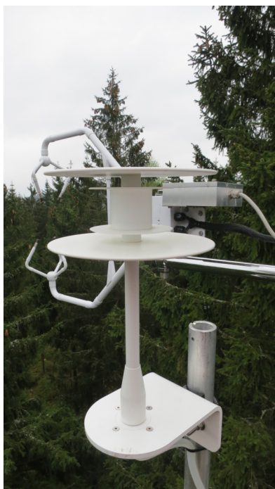
(C) Canopy measurement complex: Pressure port P2 (right) and CSAT3 S1 (left) (photo: Laura Ehrnsperger).
