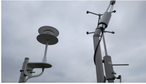
(A) Top of the canopy measurement complex: Pressure port P1 (left), Metek USA-1 S1 (in the back) and IRGA I1 (left) (photo: Laura Ehrnsperger).
