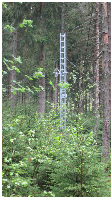
(B) Satellite station a) with sonic anemometer S5 at 4m height within the high understory vegetation.
