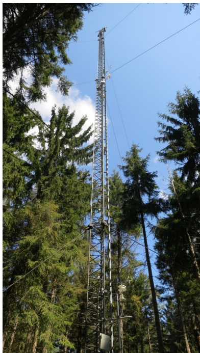
(A) Main complex with three measurement heights at the turbulence tower at Waldstein-Weidenbrunnen.
