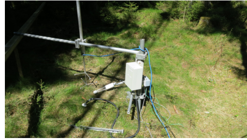
(B) Soil measurement complex with pressure transducer P4, Metek USA-1 S4 and IRGA I2 (photo: Laura Ehrnsperger).
